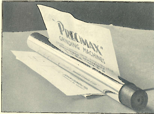
Test Bar ground on Precimax Cylindrical Grinding Machine Ovality within 0.00001, parallelism within 0.00005, mirror finish.
